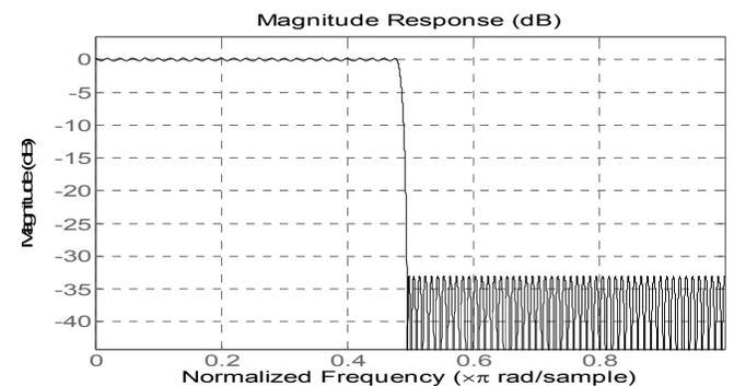
Figure 3 (b). Decimated Frequency Response of Modal FIR filter when  $M=6$ .
