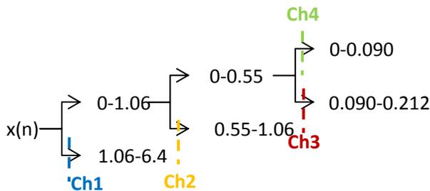
Figure 5. Proposed TNFB architecture for 4-channel channelizer in design example 2.
