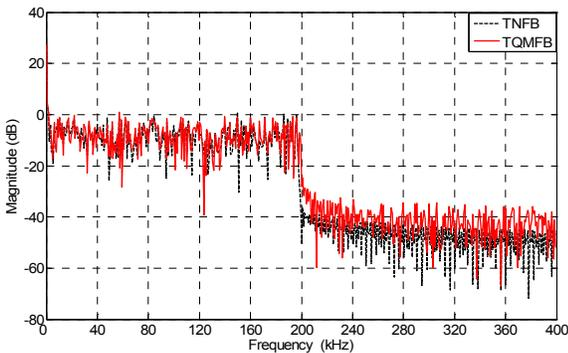
Figure 4 (b). Output response of CH1 (200 kHz) extracted using TQMF and the proposed TNFB.
