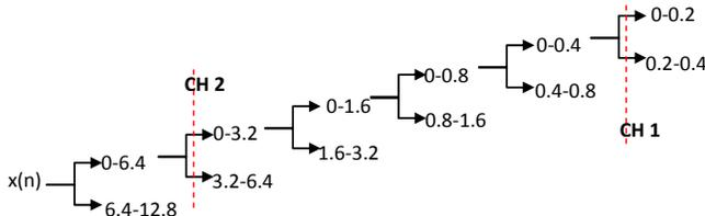
Figure 1. Tree-structure for 2-channel channelizer in design example 1.
