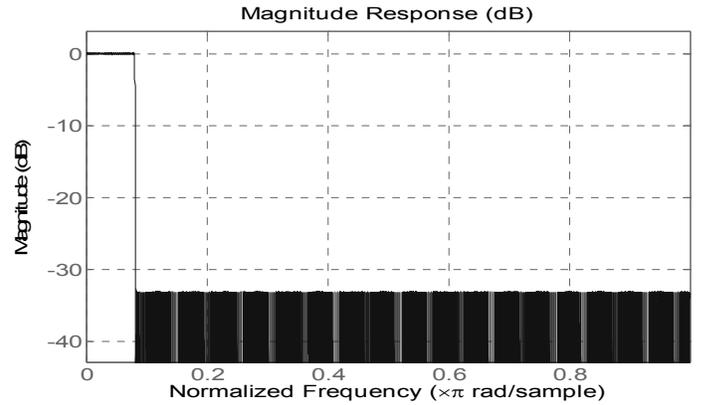
Figure 3 (a). Frequency Response of original Modal FIR filter.
