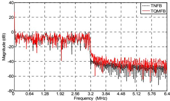
Figure 4 (a). Output response of CH2 (3.2 MHz) extracted using TQMF and the proposed TNFB.
