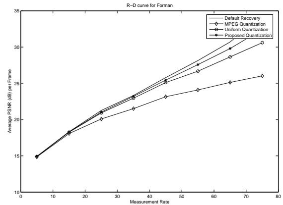
Fig. 5. Average PSNR(dB) vs. CS measurement rate for various quantization schemes using the Foreman Sequence.
