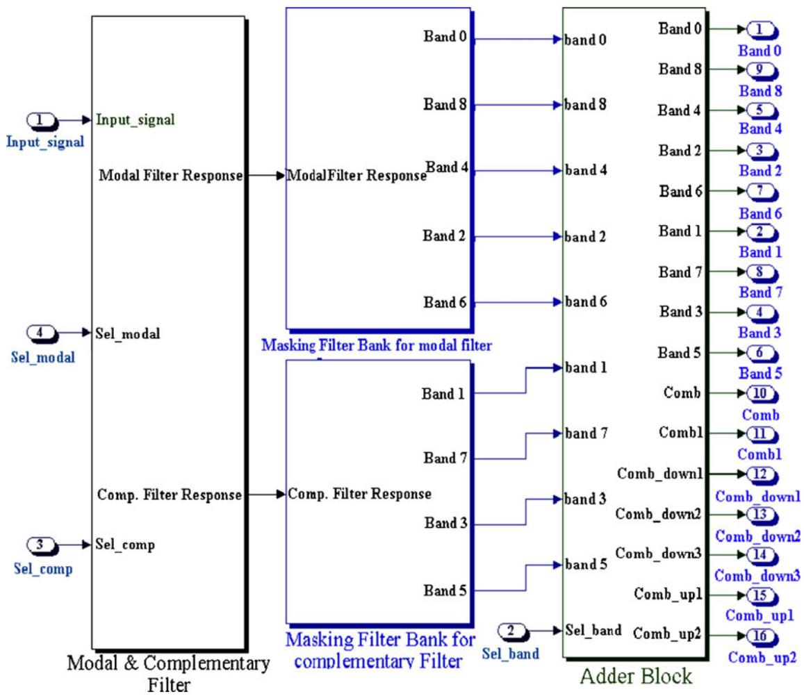
Figure 7 Three stages of FB 1) Modal and complementary filter, 2) Masking filter, 3) Adder block.
