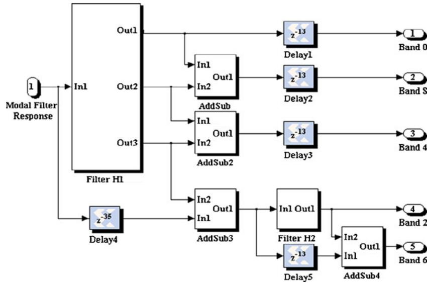
Figure 9 Architecture of Bank1 of masking filter.
