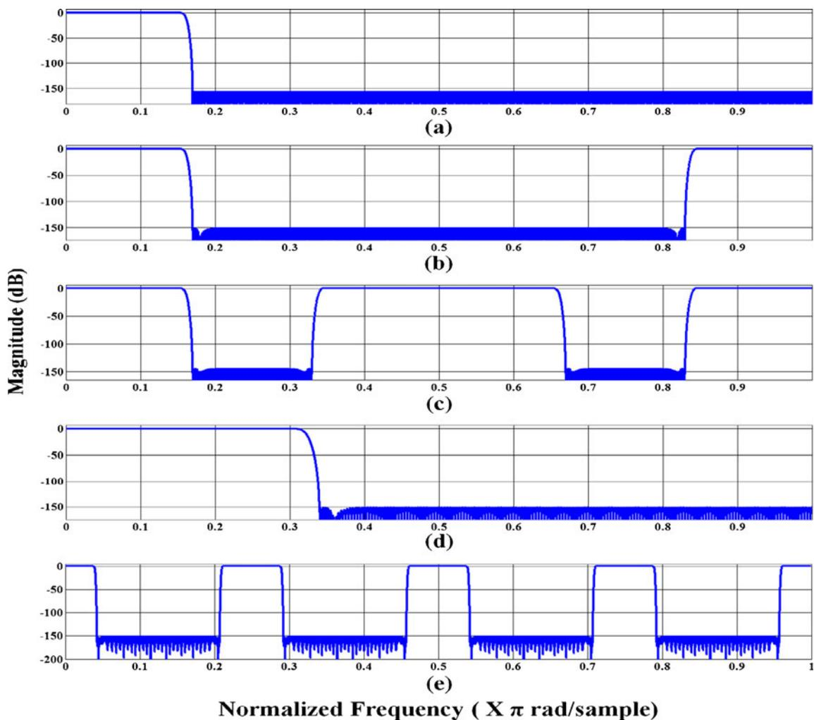
**Figure 1** a Frequency response of modal filter, b Frequency response of filter using CD-I from modal filter in (a) for  $D=2$ , c Frequency response of filter using CD-I from modal filter in (a) for  $D=4$ , d
