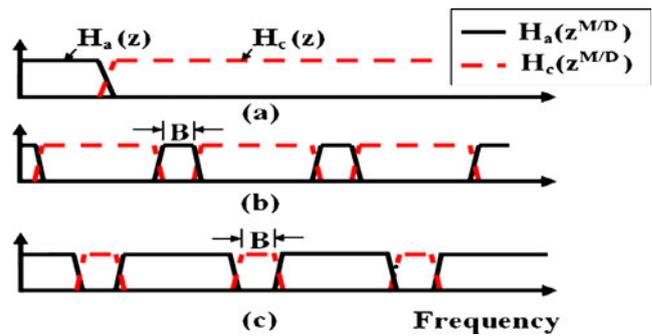
Figure 3 Frequency response showing the design of modal filter.
