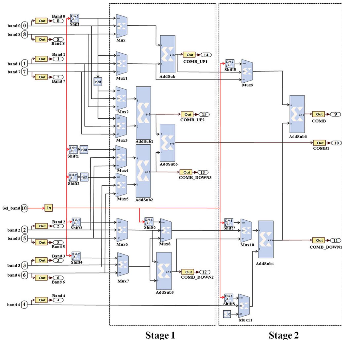
Figure 11 Architecture of Adder Block.
