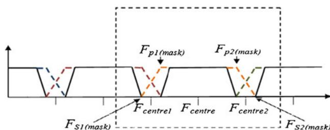
**Figure 5** Frequency plot indicating the passband and stopband frequencies of masking filter when  $D=D_{max}$ .
