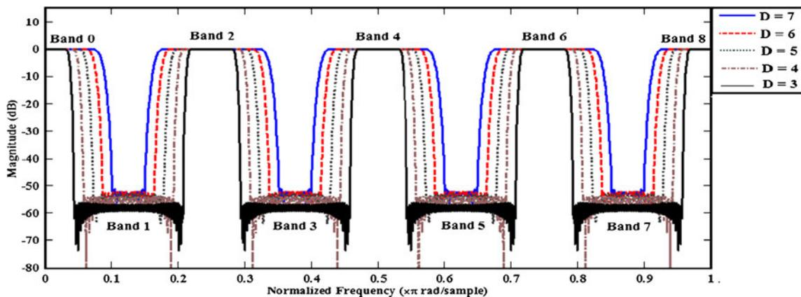
**Figure 12** Channel BW variation for modal filter with  $F_{pass}=0.083$  and  $F_{stop}=0.115$ , for different decimation ( $D$ ) factors.
