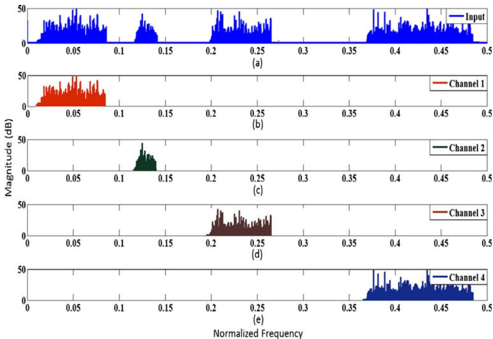
**Figure 14** **a** Input signal consisting of 6 channels, **b–g** Extracted channels 1–5 using proposed FB.
