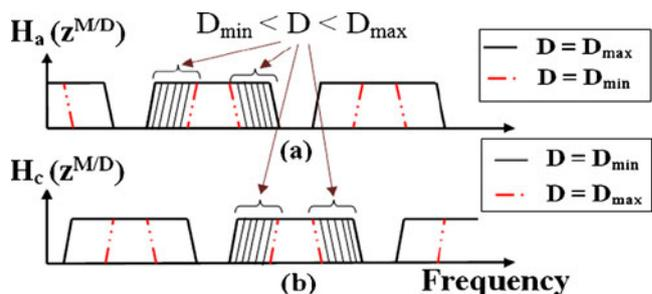
Figure 4 Frequency response of the modal filter and complementary filter for different values of  $D$ .
